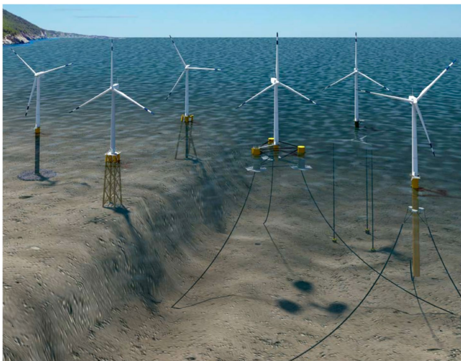
Offshore wind substructures (from left): monopile, jacket, twisted jacket, semisubmersible, tension leg platform and spar. Source: DoE.
